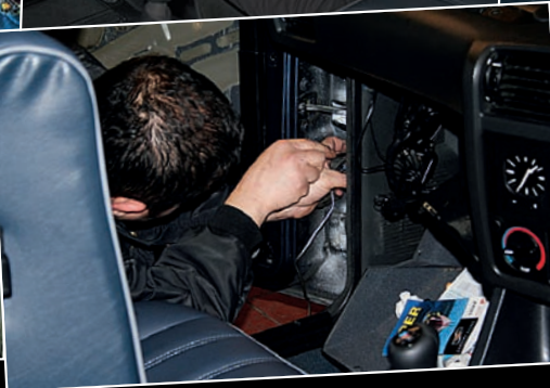
Door cards were fully stripped to wire the new Alpine tweeters to the door mirror pods, while the included crossovers separates the signal between the tweeters and mid bass drivers
