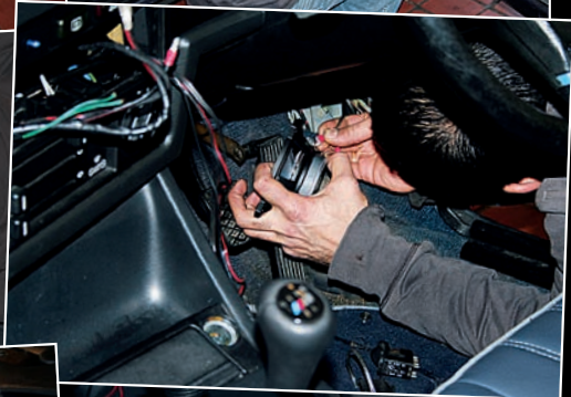
Door cards were fully stripped to wire the new Alpine tweeters to the door mirror pods, while the included crossovers separates the signal between the tweeters and mid bass drivers
