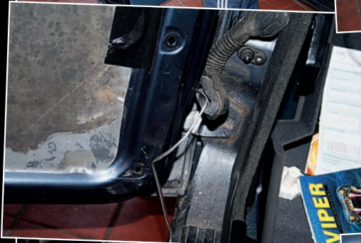
Door cards were fully stripped to wire the new Alpine tweeters to the door mirror pods, while the included crossovers separates the signal between the tweeters and mid bass drivers
