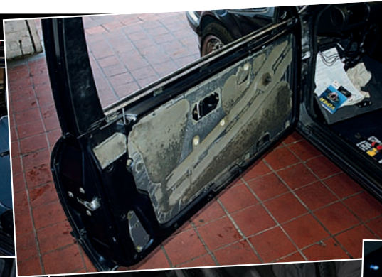
Door cards were fully stripped to wire the new Alpine tweeters to the door mirror pods, while the included crossovers separates the signal between the tweeters and mid bass drivers
